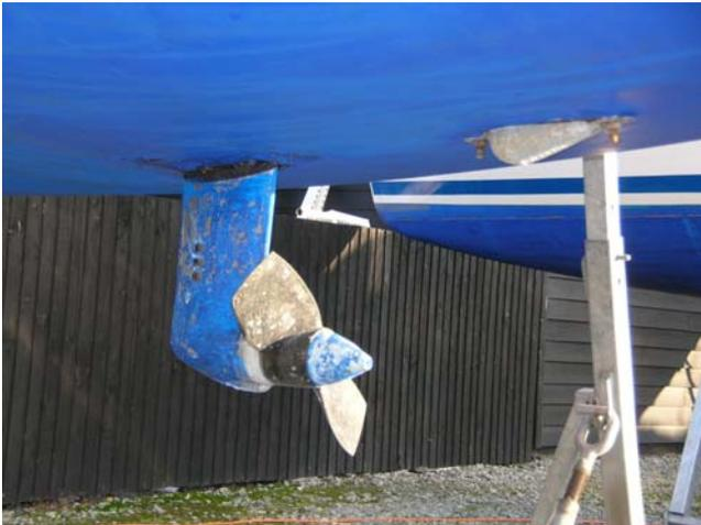
Anodes bolted onto the hull inevitably produce drag and turbulence, when the boat is moving through water. Ironically the majority of leisure boats spend less than 5% of their time afloat actually underway.
