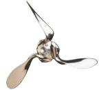
No propeller has received the research and development of Bruntons Autoprop. The world's only auto pitching propeller is now used not just on cruising sailing yachts but on displacement workboats and on the new generation of hybrid craft which are now being developed where it's unique design is ideal for maximising the available power output of the vessel.
